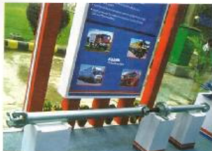
Unitised propeller shaft uses lesser number of parts. A new lightweight propeller shaft is currently under development.
